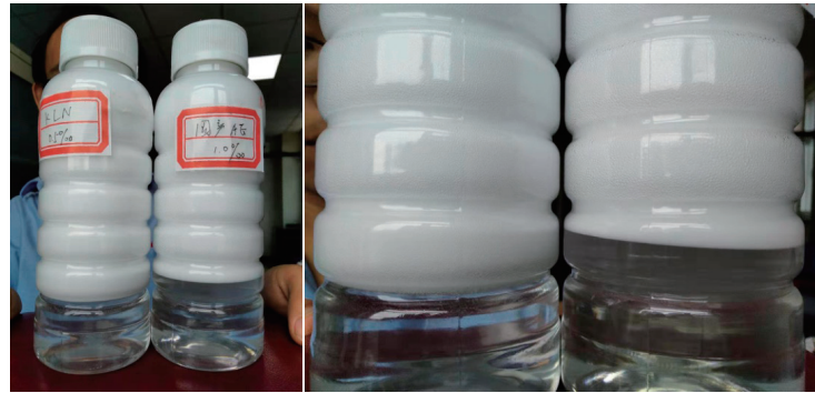
图11 气泡泡径对自由水量影响 (全图为液位比较,局部图为泡径比较,各图中左为科莱恩引气剂) Fig. 11 influence of air bubble diameter on free water (clariant air entraining agent is on the left of each)
