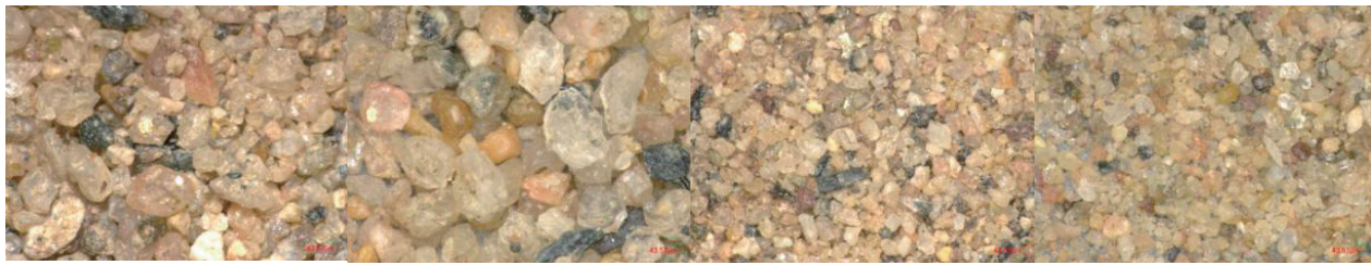
图2 河砂显微图 (从左至右依次为砂A和砂B0.15-0.3mm, 砂A和砂B0.075mm以下显微图) Fig 2 micrographs of sand A and sand B
